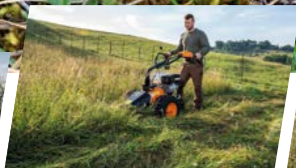
Gentle cut with double knife cutter bar
